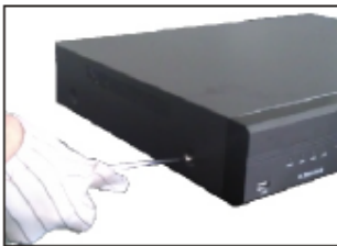
1.Tear down the fixed screws of the device top cover .
