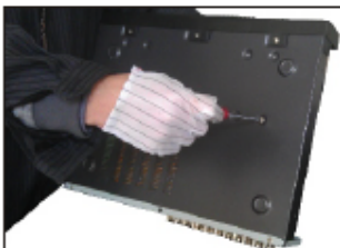
5.Fix the screws of the hard disk.
