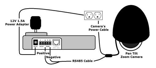
2. Power on the PTZ camera that you have connected to the PTZ controller.
