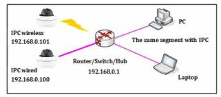
Figure 1-4 Device Connection of Network IP Camera
