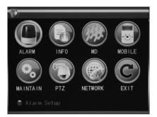
The advanced functions include the seven options of ALARM, SYSTEM INFORMATION, MOTION DETECTION, MOBILE PHONE SETTINGS, SYSTEM MAINTENANCE, PTZ SETUP, and NETWORK SETUP.
