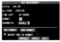
**STATUS**: After connecting the hard disk, the system will automatically detect if the hard disk is formatted. If the hard disk needs formatting, UNFORMATTED will be displayed in the hard disk state. Check the format box and select FORMAT HDD to have the DVR format the disk. If the system detects any available hard disk, the hard disk state will be ONLINE.
