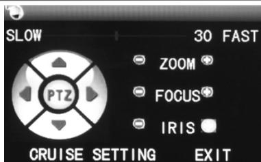
PTZ speed (fast or slow) can be controlled in this interface. Zoom, focus, and aperture are also adjustable in this menu.
